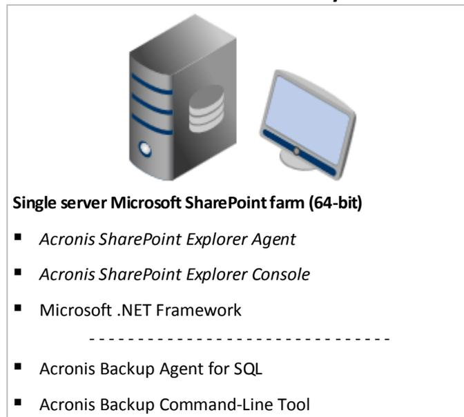
This configuration is recommended for Small Business Server solutions. This configuration enables you to extract SharePoint data from single-pass disk and application backups or from SQL databases. If one of the products shown below the dotted line is not installed, it is possible to extract data only from SQL databases.
