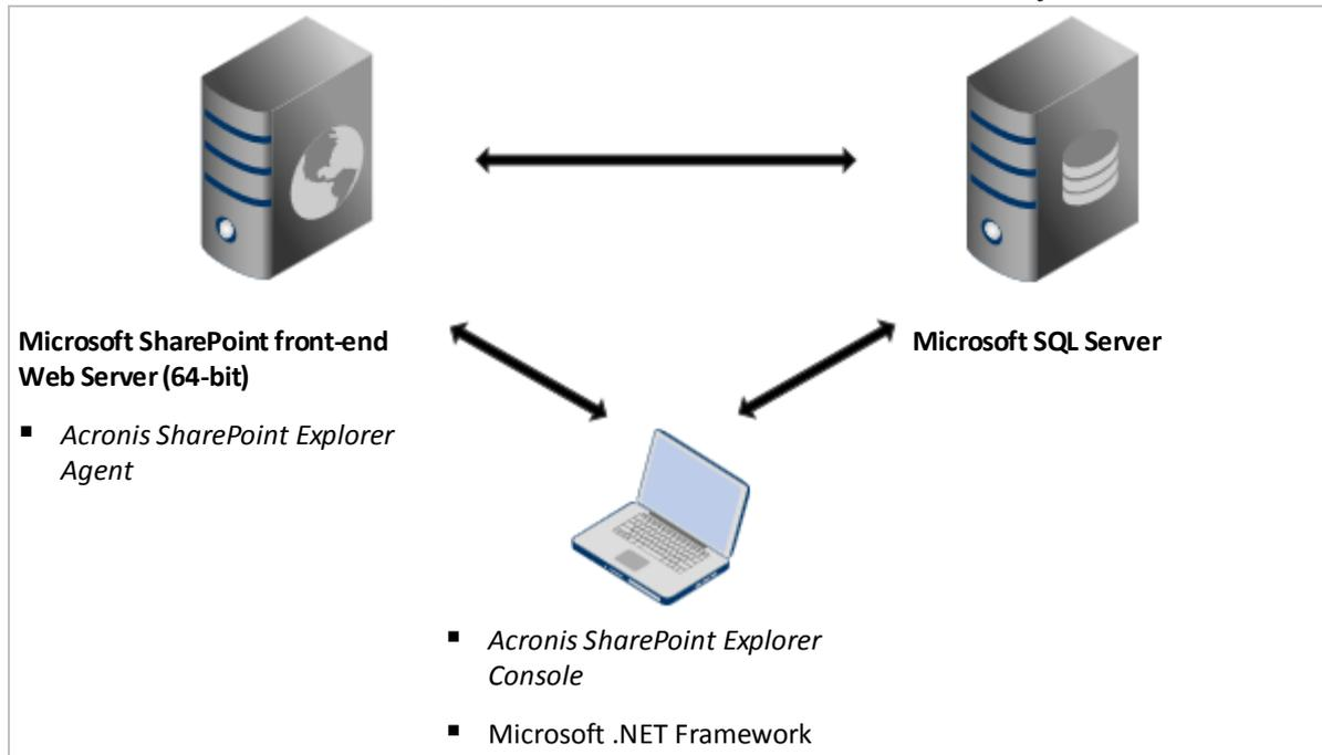
This configuration enables you to extract SharePoint data from SQL databases attached to a SQL Server instance located anywhere on the network, as long as it is accessible by both the console and SharePoint Web Front-end. Extraction from single-pass backups is not possible if the console is installed on a machine without Microsoft SQL Server.
