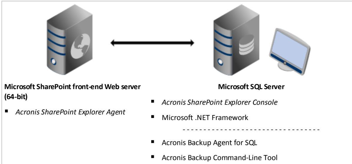
This configuration enables you to extract SharePoint data from single-pass disk and application backups or from SQL databases. If one of the products shown below the dotted line is not installed, it is possible to extract data only from SQL databases.
